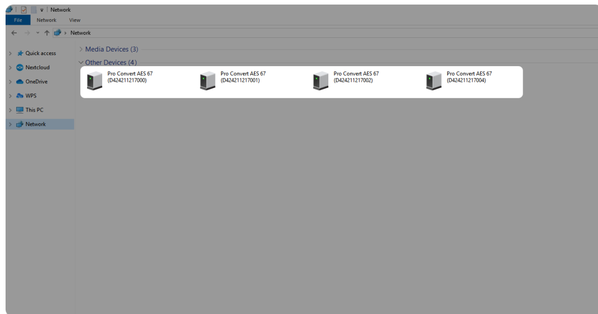
Figure2. Find your Pro Convert device in the Network > Other Devices section
